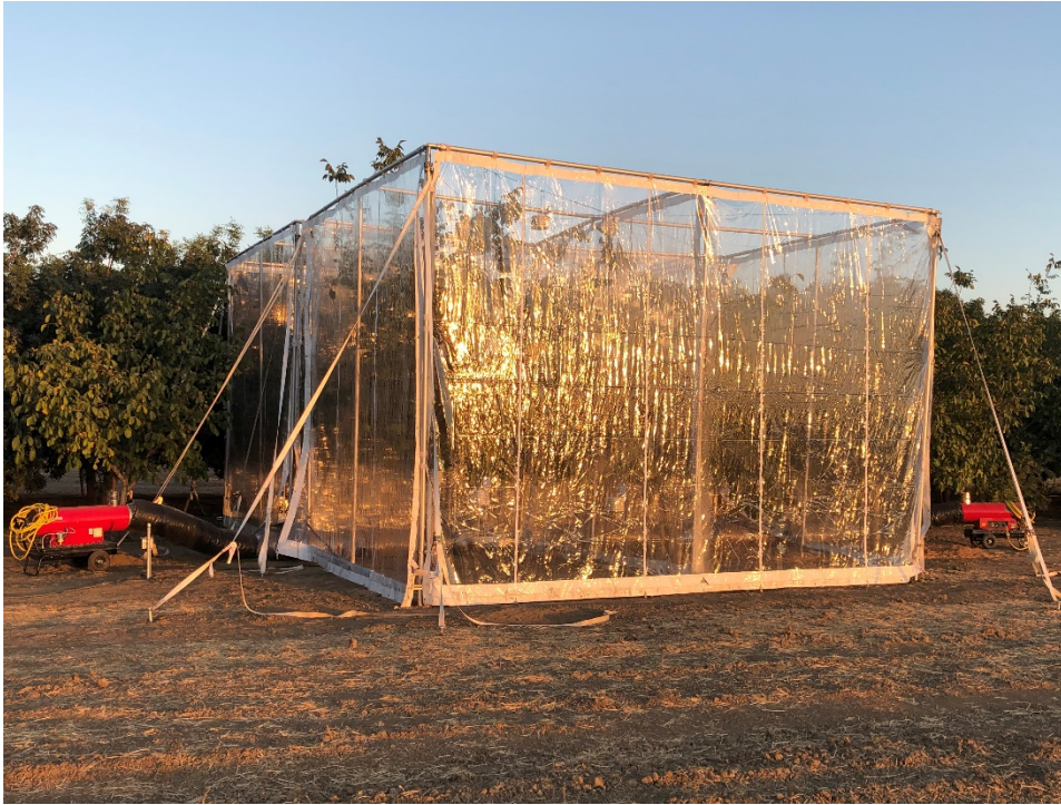
Heated Open Top Simulated Temperature Upshift in the Field (HOT STUF).
